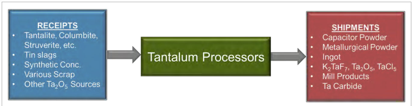
Figure 8: The general process diagram showing receipts and shipments of tantalum processors reporting to the T.I.C.
