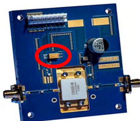
Figure 4: An example of a RF GaN power amplifier with a tantalum capacitor (circled) (photo: Cree)
