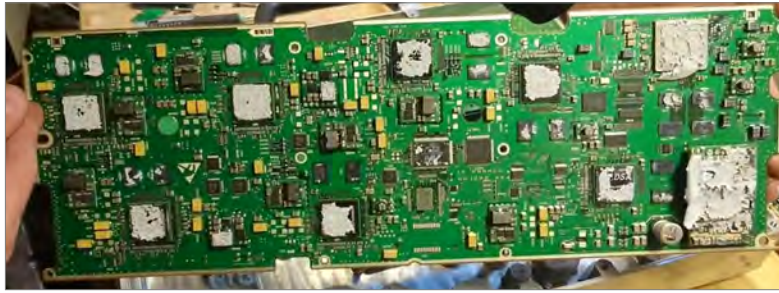
Figure 5: The design of a BS NOKIA 4G rack (~2014) carrying 35 D/E tantalum capacitors (photos: Kaizer Power Electronics YouTube Channel)
